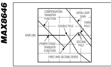
Figure 4. Type III Compensation Illustration
