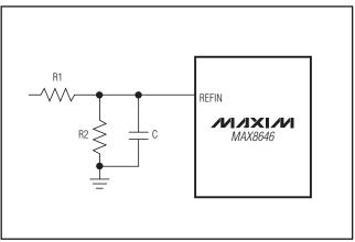
Figure 2. Typical Soft-Start Implementation with External Reference
