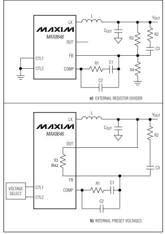
Figure 3. Type III Compensation Network
