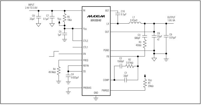
Figure 1. MAX8646 1MHz, All-Ceramic-Capacitor Design with V<sub>OUT</sub> = 1.8V
